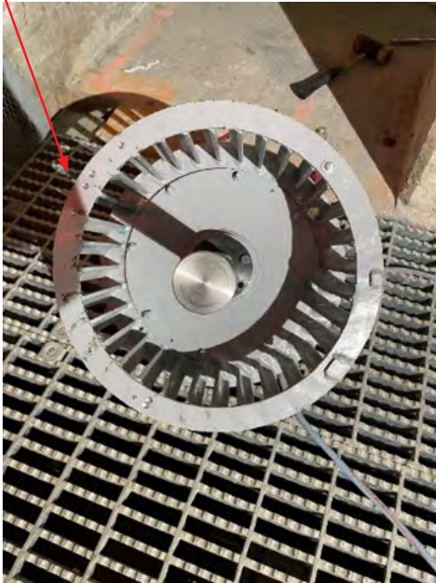
Figure 14: Brake Fan Vanes Designed with Rotation of Shaft
